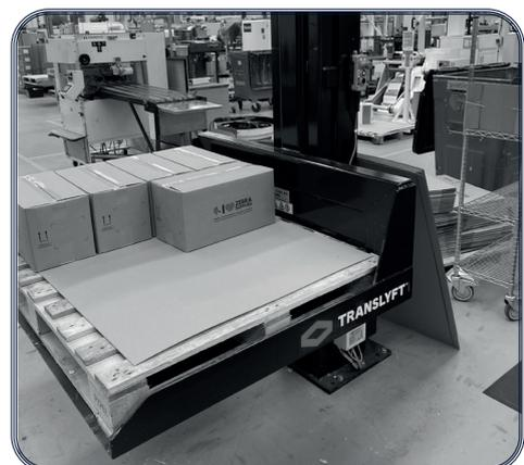
The slim design makes it easy to work besides the TSL pallet lifter and work in the most ergonomic height.
