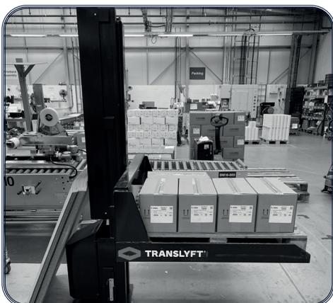
Translyft TSL pallet lifters are ideal for use in compensation for differences in work levels, in particular when used with palletized loads.
